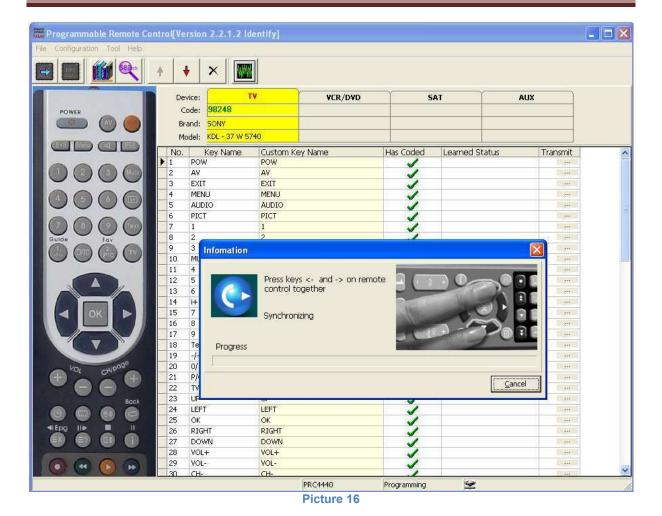
Point the programmable remote control in front of the infrared programmer. The distance should be from 1 to 5 cm.
